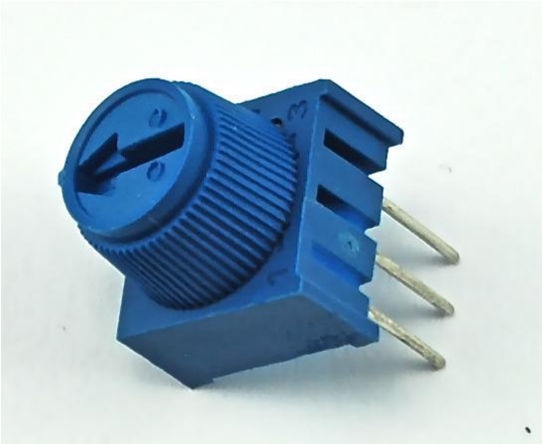
10 kΩ variable resistor (pot)
