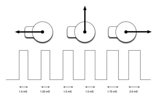
The end points of the servo can vary and many servos only turn through about 170 degrees. You can also buy 'continuous' servos that can rotate through the full 360 degrees.
