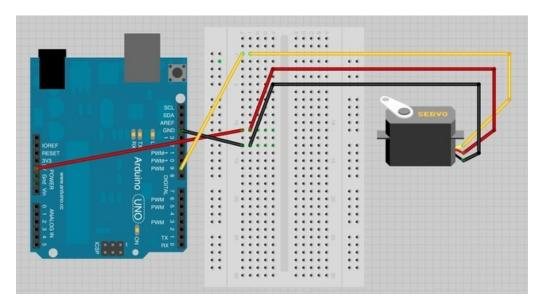
The servo motor has three leads. The color of the leads varies between servo motors, but the red lead is always 5V and GND will either be black or brown. The other lead is the control lead and this is usually orange or yellow. This control lead is connected to digital pin 9.
