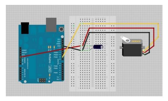
The capacitor acts as a reservoir of electricity for the motor to use, so that when it starts, it takes charge from the capacitor as well as the Arduino supply.
