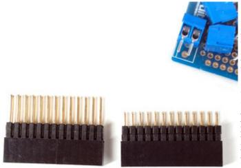
Next we will attach the header, there is a standard 'extra tall' header included in the kit. However, if you want to attach a cobbler or GertBoard, etc to the plate, you may want to opt for one of our stacking headers, they're extra long so you can plug in an IDC cable on top!
