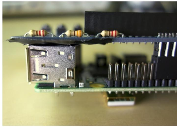
There is current limiting in the resistor circuit so it shouldn't damage the Pi if there is a short, but to be sure it is advised to cover the USB port and resistor leads in a few layers of electrical tape. Be sure to cut the resistor leads as short as possible with flush cutters and try to ensure there are no sharp edges from the cut leads or solder. See the photo below with arrows pointing to the two locations you should place electrical tape.
