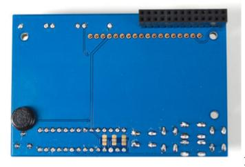
Flip over the assembly, carefully. Then solder in the 16 or 18 pins of header
