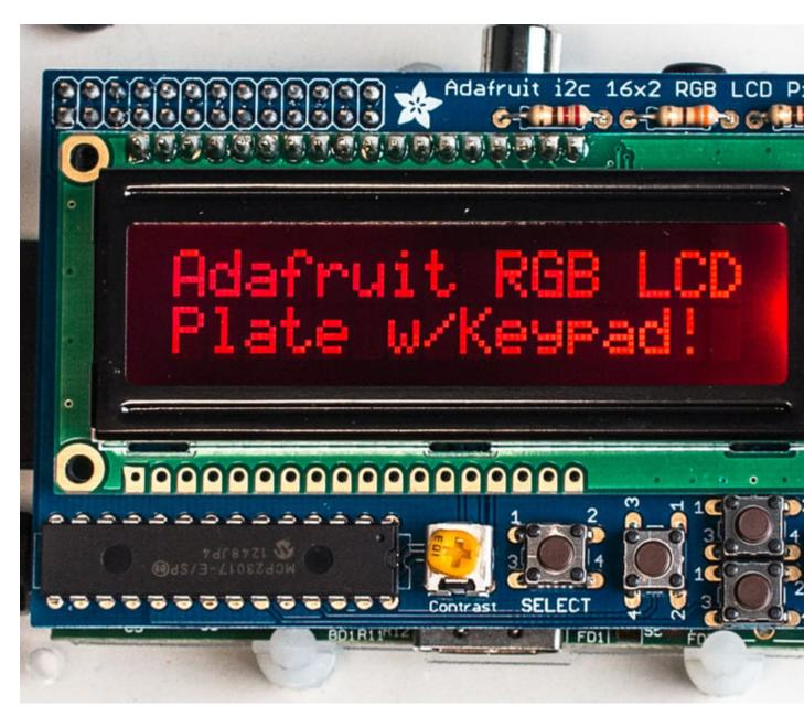
With this in mind, we wanted to make it easier for people to get these LCD into their projects so we devised a Pi plate that lets you control **a 16x2 Character LCD, up to 3 backlight pins AND 5 keypad pins using only the two I2C pins on the Pi!** The best part is you don't really lose those two pins either, since you can stick i2c-based sensors, RTCs, etc and have them share the I2C bus. This is a super slick way to add a display without all the wiring hassle.
