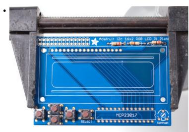
basic menu system). We have a 4-way 'direction pad' for up/down/left/right input and a button to the right called SELECT. These 5 buttons should be able to make 'talking' back to your project easy. These are connected to the I2C port expander chip so they require no extra pins on the Pi, our library does the work of reading whether they are pressed.
