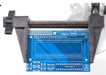
This resistor acts as the backlight control resistor for the green backlight pin.
