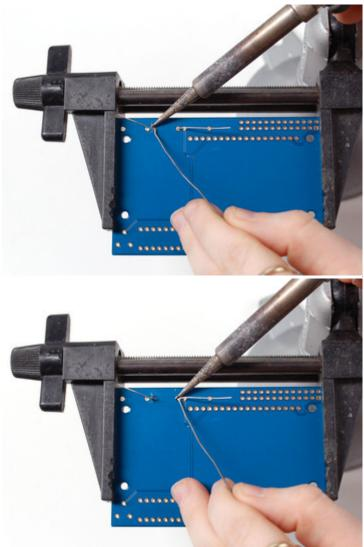
Bend the 'legs' of the resistor out so it sits flat against the PCB and flip it over.
