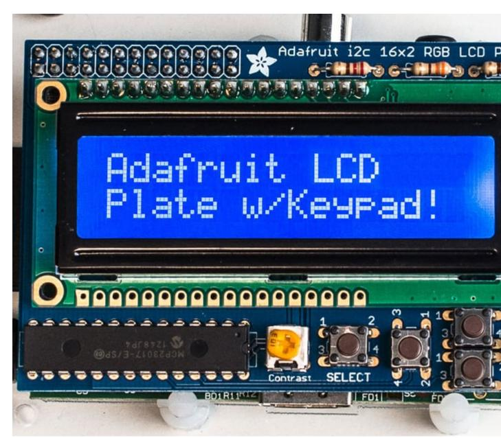
WARNING: The new Raspberry Pi model B+ with 4 USB ports overlaps closely with backlight resistor leads on the char LCD plate. You will need to cover the USB port and back of resistors with electrical tape to protect them from touching. See more details and pictures on the assembly page of this guide.
