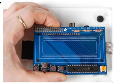
Place the 2x13 header onto your Pi, and slide the plate on top, it should fit perfectly.
