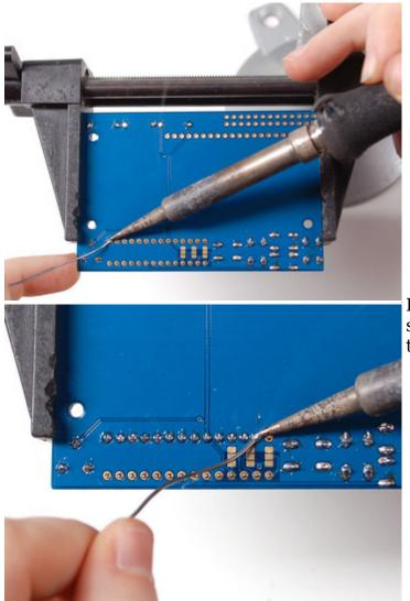
Flip over the PCB and solder in the 28 pins of the port expander.
