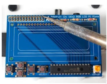
Now we will solder all 26 pins for the plate - this will send power and data between the two boards and also provide a mechanical stability. You may need to hold the plate down with tape to get it sitting flat against the Pi.
