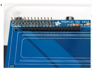
Finally, we place the LCD. Break off a piece of 18 or 16 pin header from the stick in the kit.
