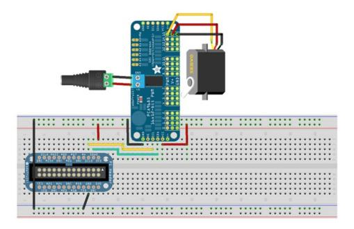
VCC = the digital supply for the IC (3.3V!), V+ = the supply for the servo motors (typically 5V). Be sure not to confuse the two or you may end up with burnt Pi!
