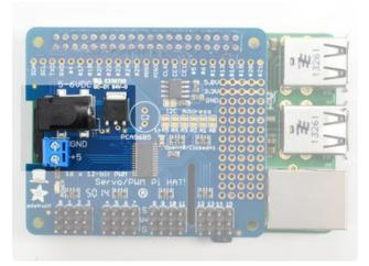
The power input section of the HAT and Bonnet are both on the left hand side.
