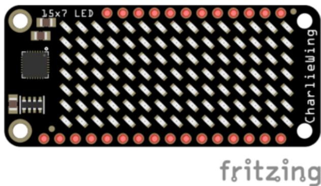
Assemble the CharlieWing by soldering headers onto the board. Once assembled, plug it into a Feather!
