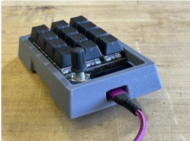
Access the **STEMMA QT I2C** port and the **reset** button from the left side of the case.
