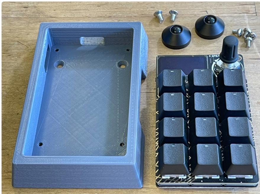
Follow the basic instructions for [MacroPad assembly \(https://adafru.it/TOF\)](https://adafru.it/TOF) in the main guide -- but don't attach the back plate. Switch plate, keyswitches, encoder knob, keycaps, and the MacroPad itself should be assembled first, as shown above.
