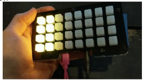
The 'grains of sand' code is a great way to demo any LED matrix with an accelerometer, and the NeoTrellis M4 can make this even more entrancing by adding tactile, tap, and sound interaction as well.
