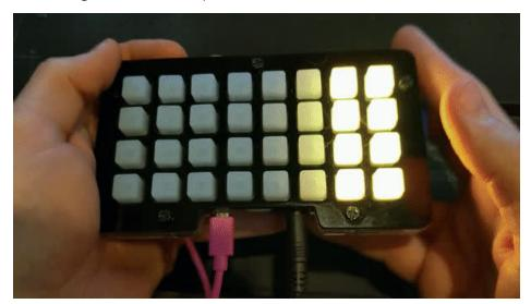
In the solid color mode, pushing any button on the NeoTrellis will rapidly change the color randomly. You can hold down for a random color effect, or quickly press to change to a new random color.
