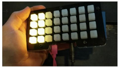
A sharp 'tap' anywhere on the NeoTrellis will switch the color mode - there are three modes built in:
