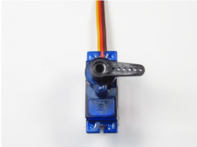
Hold the servo so the end with the wires is facing up when you are looking straight down at it. Press the one-armed horn (also called a half horn) onto the shaft of the motor so it is pointing to the right (three o'clock position).
