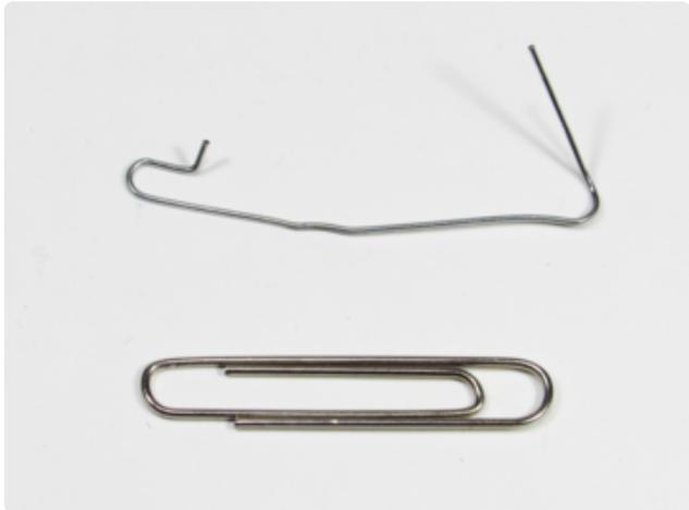
Unbend a paperclip in the middle and straighten it out. The larger end will go towards the front.
