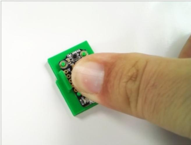
Firmly press the Trinket M0 onto the backplate.
