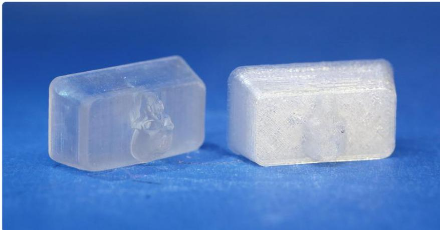
With that said, the keycaps can print just fine on FDM printers. Translucent PLA colors aren't completely see through. As layers get stacked on top of each other, objects will start to look more opaque . We definitely recommend using SLA for higher quality prints, especially if you want the see through look.
