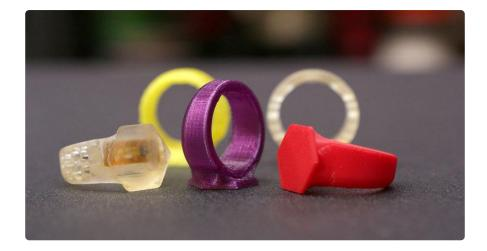
In this project we're embedding an RFID tag into a 3D printed ring.
