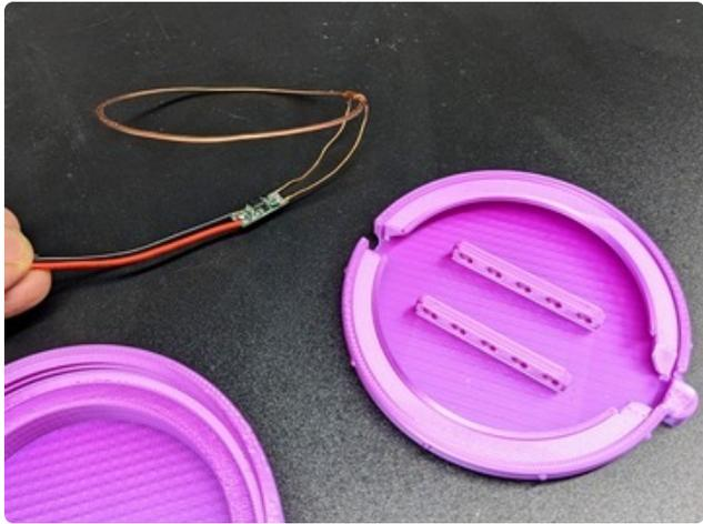
To make the power transmitter fit inside the holder, you must gently bend the power wires back underneath the coil as shown. Don't crease the wires sharply and keep about 1 cm separation between the two wires leading from the coil.
