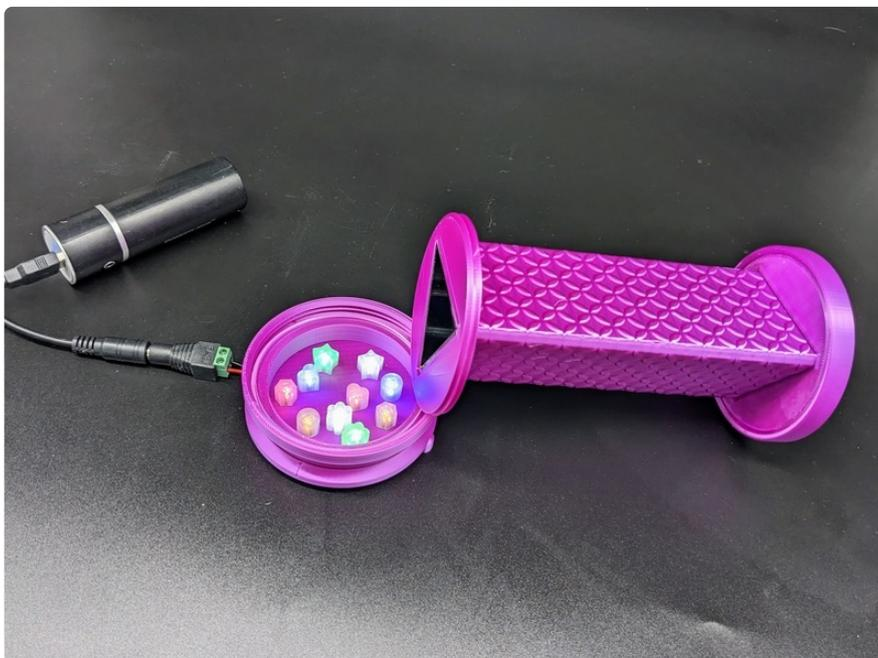
Gently rotate the body of the kaleidoscope until the eyepiece and LED container threads mesh, and the eyepiece moves down into the container. Stop turning just when the eyepiece touches the lens. Do not overtighten.
