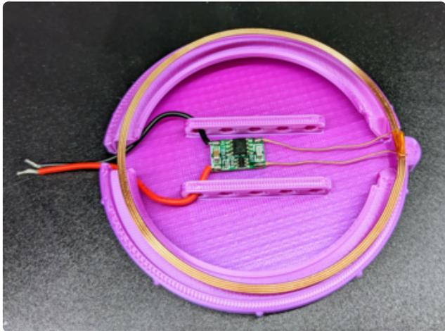
Place the coil inside the coil holder compartment as shown as left. The coil should rest inside the elevated ring, and both the black and red power wires should run through a hole in one of the interior rails to protect the electronics from strain on the wires. The ends of the wires should extend outside the compartment through the hole in the side opposite to the small exterior knob.
