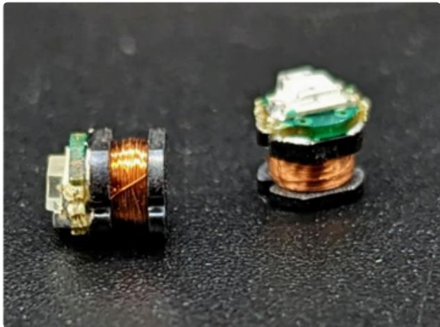
Looking closely at the tiny lights reveals that each is attached to a small assembly of tightly coiled magnet wire. Power is transmitted to these coils using principle known as **Faraday's Law of Induction**, which states that changing magnetic fields generate electric current, and also the converse, that electric current generates a magnetic field.
