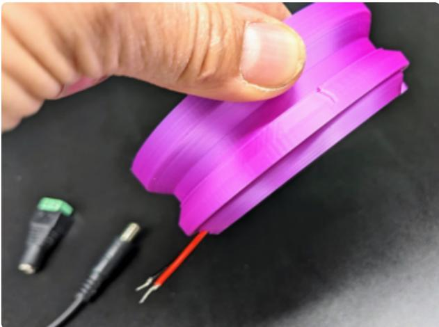
Once they have fully snapped together, you should be able to slide the bezel and coil holder together so that they rotate around the LED compartment freely.
