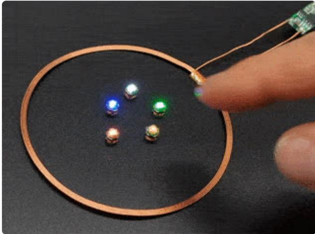
Additionally the orientation of the receiving coils and transmitting coils must be parallel. You can experiment with your wireless LEDs by placing the LEDs and transmitting coil on a flat surface, and providing 5V power to the induction coil. Notice that turning the LEDs on their side stops them from lighting up.
