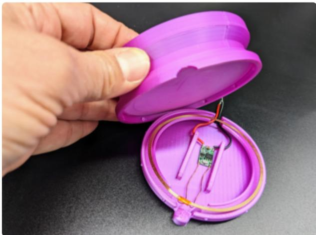
Place the LED compartment over the coil holder. Push down the bezel so that it extends past the bottom of the LED compartment, and orient the bezel so that the notch aligns with the knob on the coil holder. Be sure the power wires extend out of the hole in the side of the coil holder.
