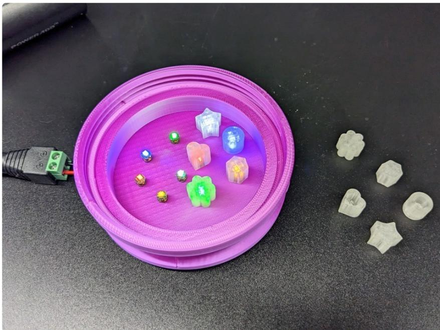
Once you've covered all of the LEDs, place the second acrylic lens over the top of the LED compartment. The small clearance between the lens and the LED covers will let them slide around while still maintaining the orientation of the LED coils parallel to the transmitting coil.
