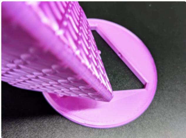
Insert one end of the triangular body into the triangular hole in the eyepiece. The three small bumps on the end of the triangular body fit inside corresponding notches in the eyepiece, and a bit of gentle pressure will help slide it into place.
