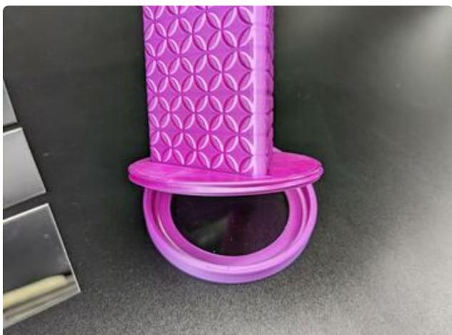
Once the body and eyepiece click together, set the eyepiece cover on a flat surface with its screw threads pointed upwards. Remove any protective paper from one of the 3" clear acrylic lenses, and place it inside the eyepiece cover.
