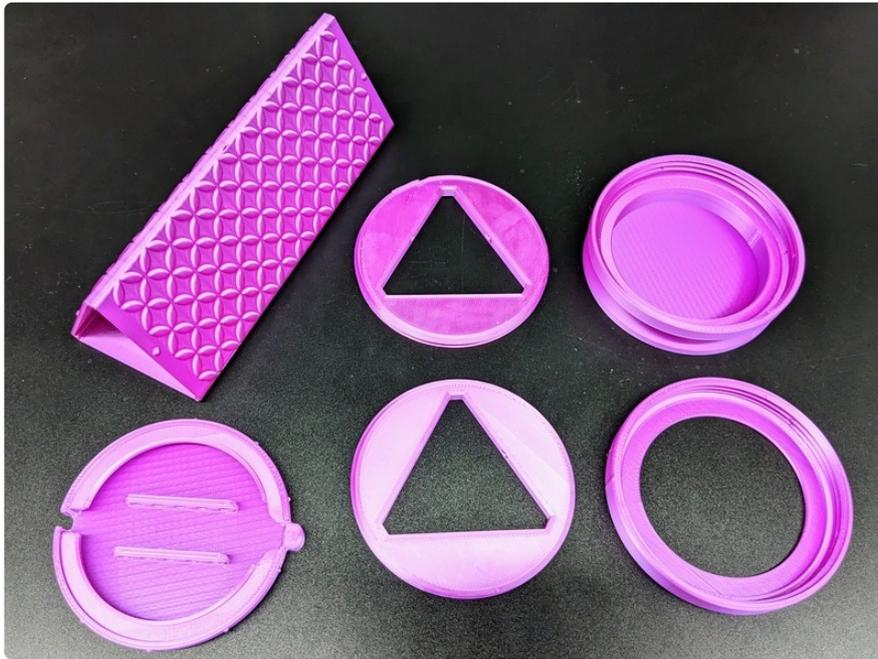
Import the STL files into the slicer program for your 3D printer. The designs include fine detail like screw threads, and should be printed at fairly high resolution to function well. A **layer height of 0.2mm with 40% infill and no support** works well for all kaleidoscope body parts.
