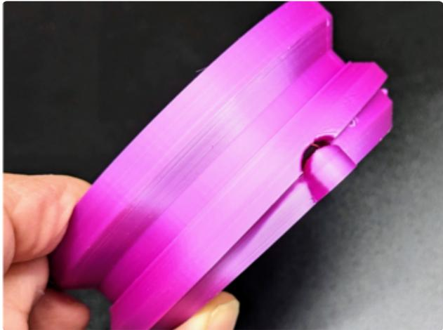
Press the bezel down over the coil holder so that the bumps in the holder slip into the small notches on the bezel interior. The knob in the coil holder will fit into the large notch in the bottom of the bezel. You may need to push the two pieces together incrementally, working your way around the circle as you go.
