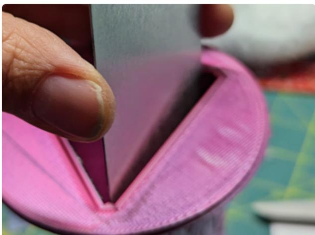
Peel the protective covering from the shiny side of the mirror. After this point, try avoid touching the mirror surface, instead, hold the mirror pieces by their edges. Next, peel the paper covering the adhesive back surface of the mirror, and gently slide it inside the kaleidoscope body until it fits fully inside.
