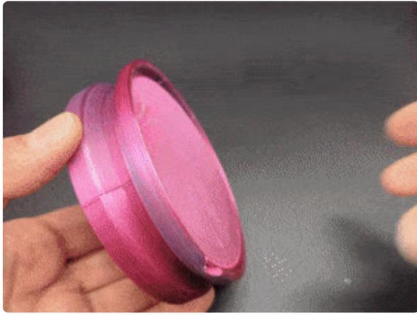
Note that the LED holder is technically two separate pieces that print together so that the bezel is free to rotate around the exterior of the LED compartment, but can't slide off the top or bottom. This **MUST** be printed as a single piece with the same positioning as in the LEDContainerWithBezel.stl file.
