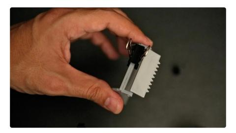
Once dry, slip the belt end under the teeth of the latch and pull back to grip on tight.
