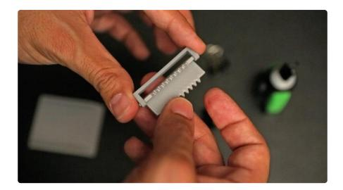
We used super glue to bond the bottom part to the base. Make sure to glue with the teeth facing towards the inside of the base with the bevels on the side as soon below. Use two small binder clips to hold the pieces together while they dry.
