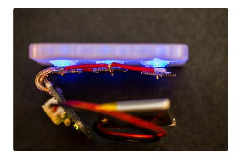
The diffuser and all of the components easily fit inside the cavity of the buckle cover. With full circuit powered on, snap the lid onto to the back of the buckle cover. Now snap in the buckle cover onto the base. The buckle should fit up to 42mm wide canvas belts. The teeth on the latch and buckle cover tightly grip onto the canvas and securely fit onto your waist.
