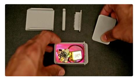
To snap the cover on to the base, slightly pull back one of the sides and pop each nub into place.
