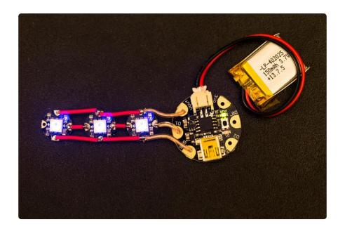
Once you have your wires measured, cut and stripped, wire them together to test the circut. Test your connections before soldering all of the connections to Gemma by connecting the small LiPo battery to the power port. Use pieces of paper tape to hold the strand of NeoPixels onto the diffuser. The Gemma should have enough wire to fold over the strand of NeoPixels, as shown in the photo below.
