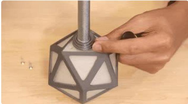
We need to secure the head of the mace to the d2m-led.stl part using 4x 4-40 (3/8 long) machine screws. Insert one screw into the one of the holes on the bottom of the part and use a screw driver to fasten the screw until goes through the d2m-led.stl and d2m-shell.stl.
