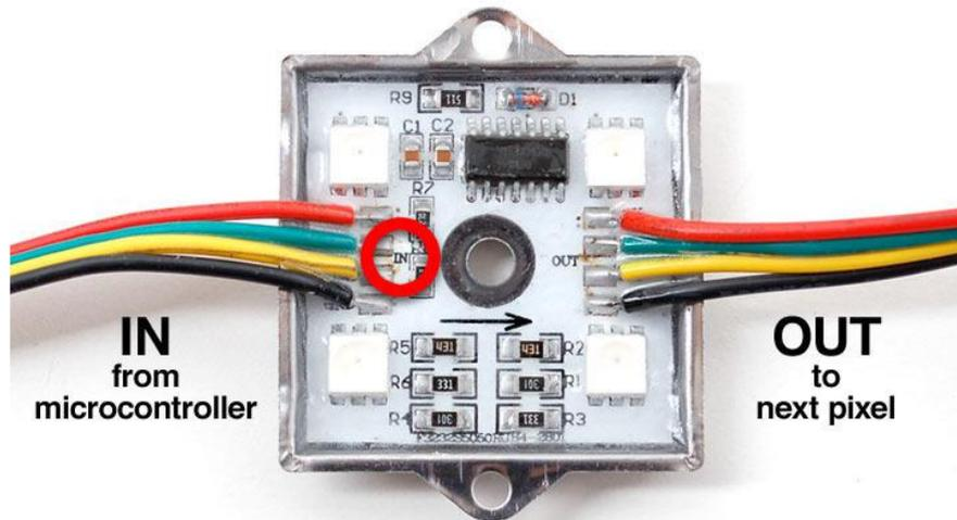
The pixel strands include plugs for joining multiple strands, plus two wires for connecting power:
