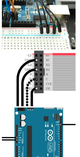
**32x32** and **64x32** matrices require **three** ground connections. **32x16** matrices have **four**.
