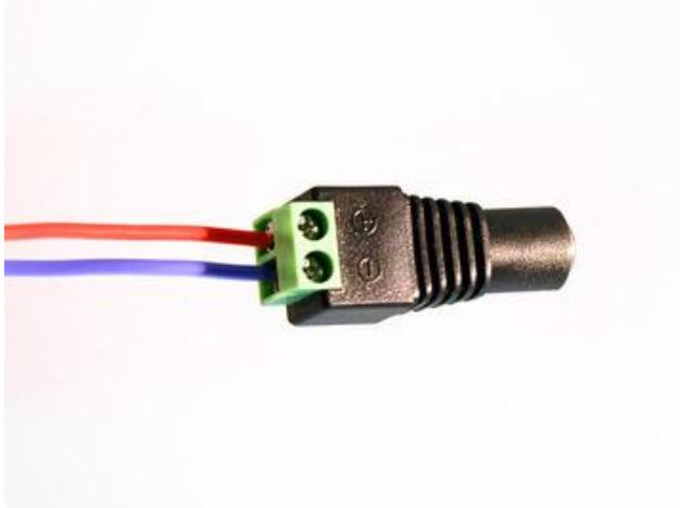
The [female DC power adapter \(http://adafru.it/368\)](http://adafru.it/368) mates with either of the above power supplies. Screw terminals clamp down on the power leads at the end of a strand, reducing the amount of soldering required.
