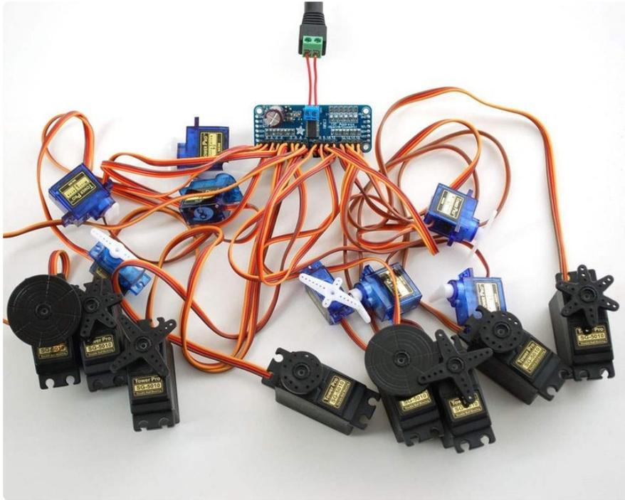
Driving servo motors with the Arduino Servo library is pretty easy, but each one consumes a precious pin - not to mention some Arduino processing power. The Adafruit 16-Channel 12-bit PWM/Servo Driver will drive up to 16 servos over I2C with only 2 pins. The on-board PWM controller will drive all 16 channels simultaneously with no additional Arduino processing overhead. What's more, you can chain up to 62 of them to control up to 992 servos - all with the same 2 pins!
