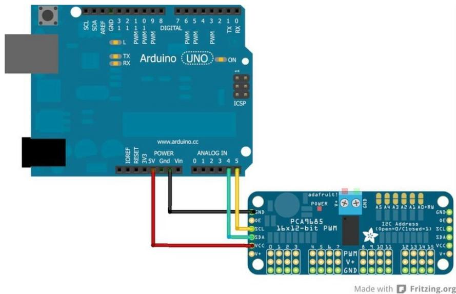
The VCC pin is just power for the chip itself. If you want to connect servos or LEDs that use the V+ pins, you MUST connect the V+ pin as well. The V+ pin can be as high as 6V even if VCC is 3.3V (the chip is 5V safe). We suggest connecting power through the blue terminal block since it is polarity protected.
