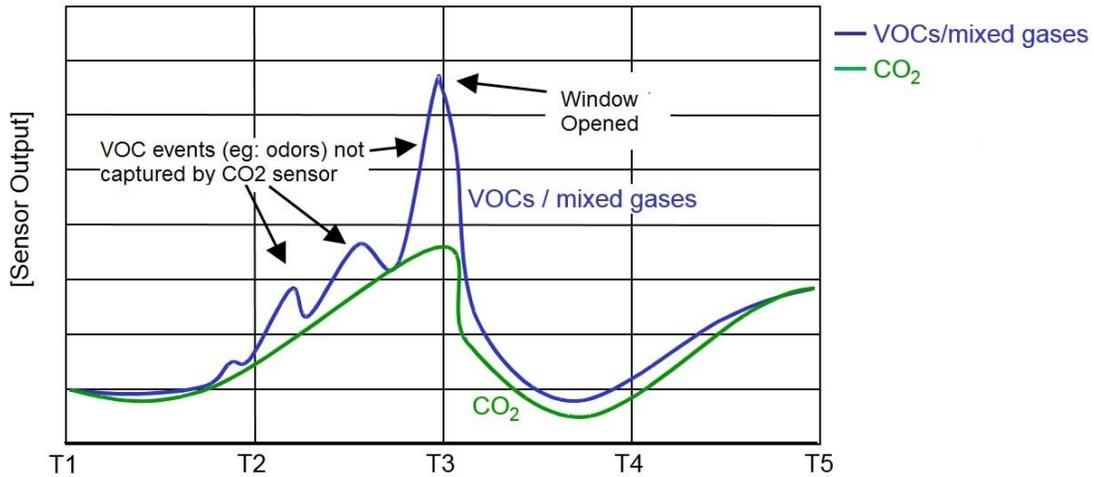
Time vs. CO<sub>2</sub> Sensor and Scaled Relative VOC Level response to ambient air in a meeting room
