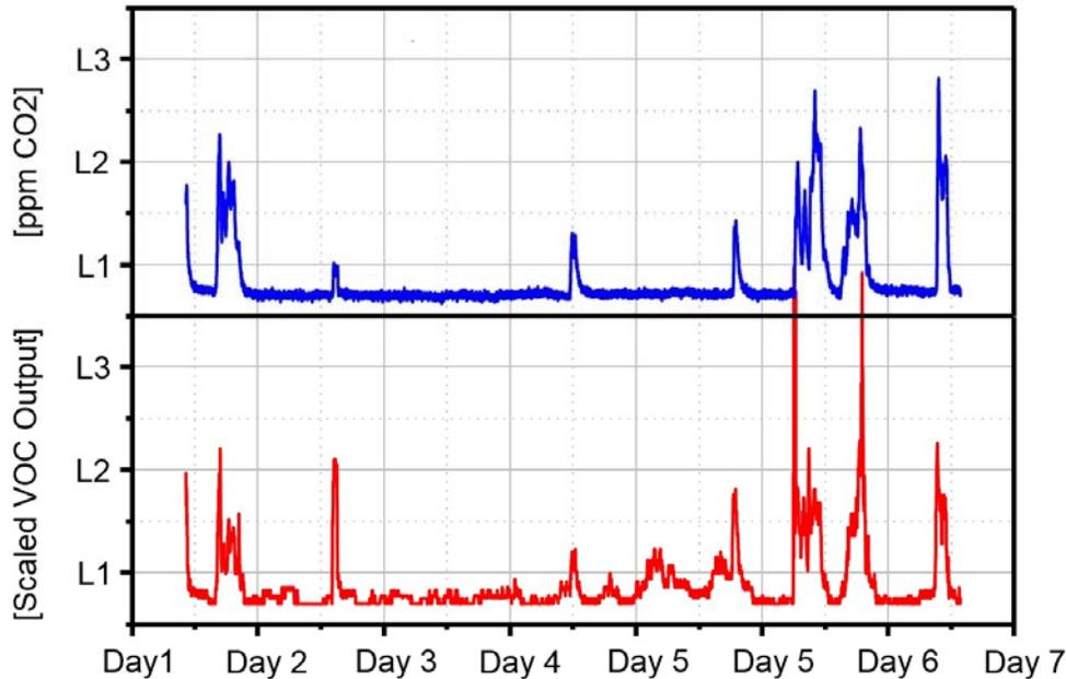
Fig. 4: comparison of calculated, scaled eCO<sub>2</sub> values from an ams MOX gas sensor with actual values measured by an absolute CO<sub>2</sub> sensor over a seven day period
