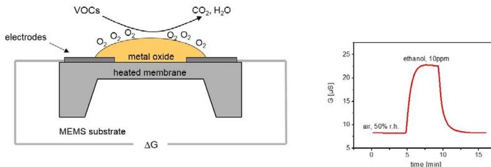
**VOC Sensor Operating Principle with Sensor Diagram and Example Response to VOC**
